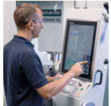
When machining in CNC mode, all advantages of a 3-/4-axis CNC machine are available. The workshop-oriented digital Heidenhain TNC 620 controls can be programmed in conversational mode (Heidenhain plain text) or via DIN ISO. A large number of graphically supported cycles are available for the most common operations (pocket machining, grooving, zero-point shifting, etc.). Of course, programs created by CAM can also be transmitted directly to the controls.
