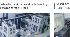
Linear automation solution consisting of two VERSA 825 with rack magazines for up to 346 tools each
