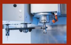
The tool changer is integrated in the machine to save space. Tools are automatically changed by means of a double gripper. Depending on the version, there is space for 20 or 30 tools in the magazine.
