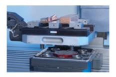
The workpiece feeding system with pallet handling is perfectly suited for medium-sized batches and single parts. Various clamping devices may be mounted on the pallets without having to program a robot.
