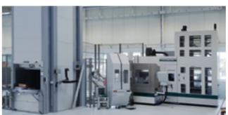
Articulated arm robot system for blank parts and pallet handling on VERSA 825 with rack magazine for 346 tools
