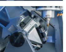
With the VERSA 745, workpieces up to Ø 500 mm can be precisely machined in 5 axes. The rotary tilting table is integrated along the X-axis and has a generous swiveling range of  $-135^{\circ}/+120^{\circ}$ . The gray cast iron construction, the thermo-symmetrical design and the fact that only two axes on the tool side are used for cutting result in high rigidity and precision, as well as maximum dynamic accuracy.
