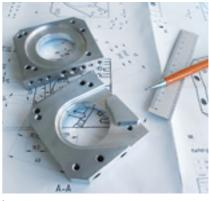
Removing residual material by milling, adding holes and threads or easy and fast machining of fixtures all based on a CNC program: With its TOP and mill functions, the PICOMAX 56 offers both the advantages of a manual and a CNC machine. Manual operation at the touch of a button.
